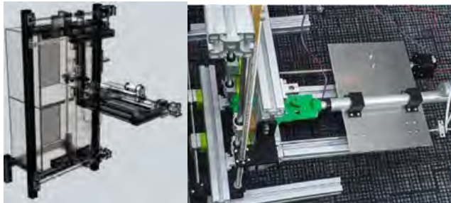
Design using MOI3D (left) & Actual developed product (right)
