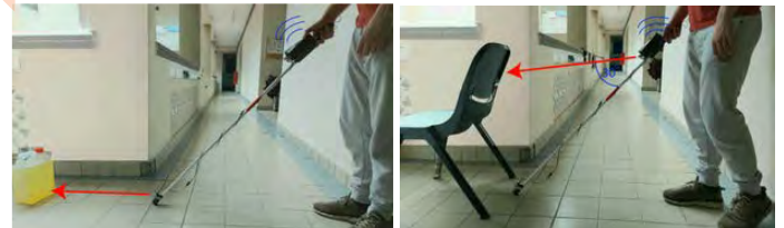
Obstacles are placed below and above of the user's knee to determine the efficiency of the proposed Smart Cane
