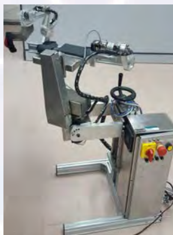
Robotic exoskeleton with assist-as-needed control
